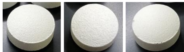
Fig. 1. Image of tablets coated with (left to right): Opadry® II, Opadry® TF calcium carbonate and Opadry® TF rice starch.
